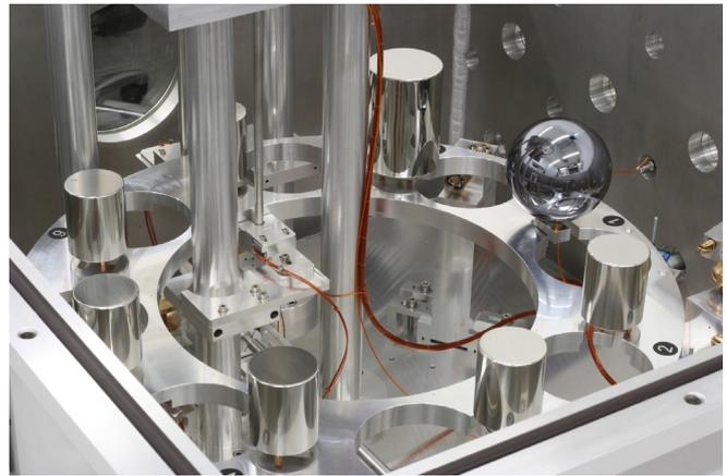
**Fig. 3. Integrated turntable with eight positions**
