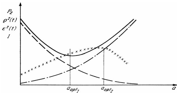
Fig. 2. Errors and information flow as a function of the degree of correction
