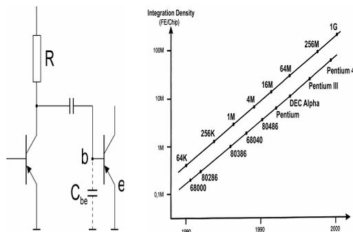
**Fig. 1. Left hand side: Typical circuit (amplifier) with the decisive base-emitter-capacitance  $C_{be}$
