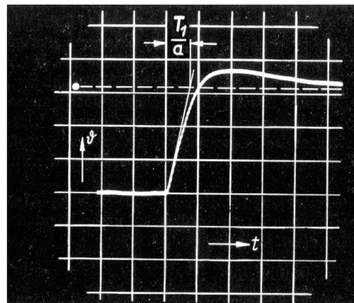
Fig. 4. Influence of a difference between the time constants of the original and the correcting system  $\Delta T = +0.2$  (parameter sensitivity)
