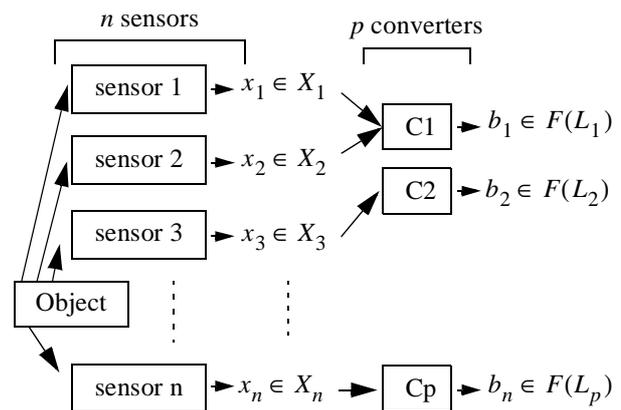
Fig. 3. Structure of a fuzzy sensor
