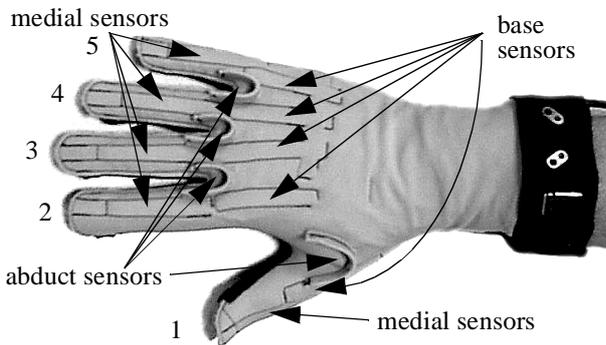
Fig. 2. Picture of the cyberglove, name of the sensors and fingers numbering
