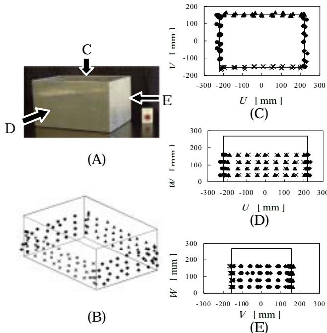
Fig.7 Result of recognizing four side faces of rectangular parallelepiped
