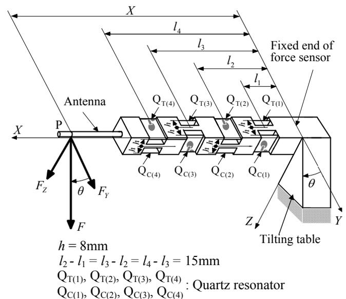
Fig. 1 Outline of experimental antenna with force sensor using four pairs of quartz resonators
