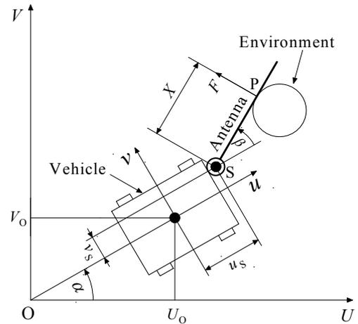
Fig. 5 Coordinate systems for active antenna
