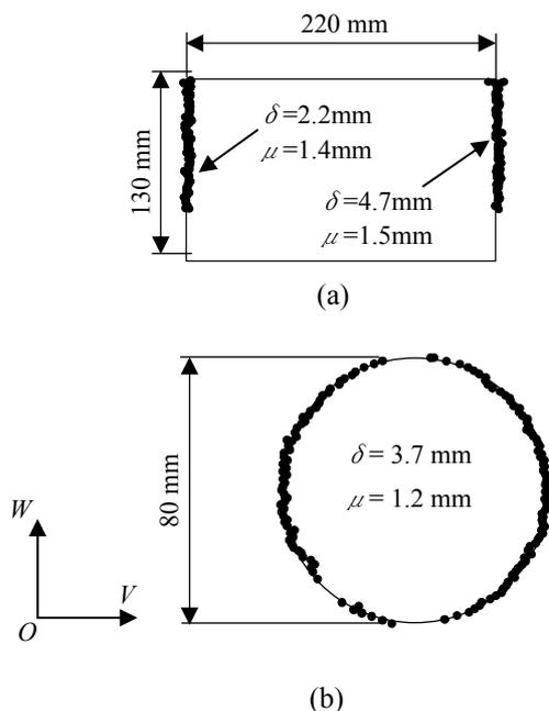
Fig.6 Result of recognizing (a) both sides of a rectangular plate and (b) outer periphery of circular plate
