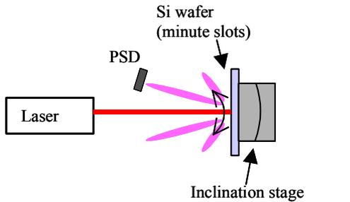
Fig.4 Angle measurement experiment
