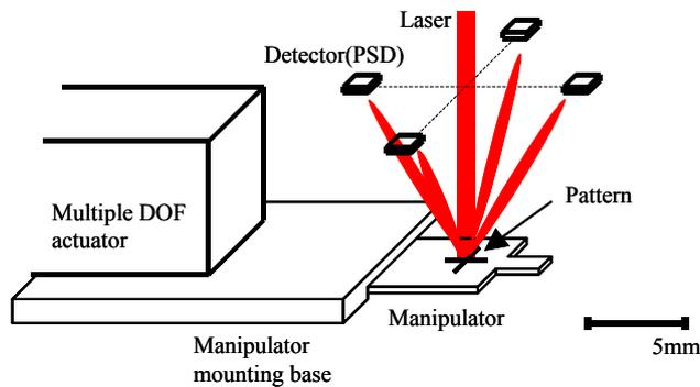
Fig.2 Schematic diagram of instrumentation
