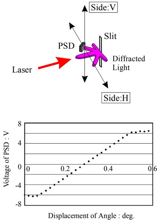
Fig.5 Angle displacement measurement precision
