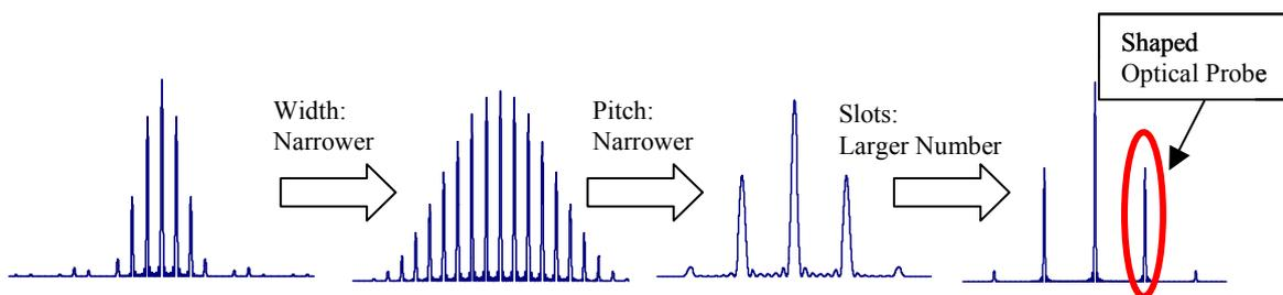
Fig.8 Effect of selected parameters to distribution of diffracted light
