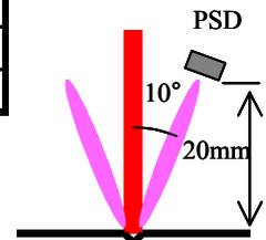
Displacement of spot position on PSD
