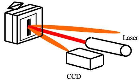
Fig.11 Experimental device for horizontal displacement measurement
