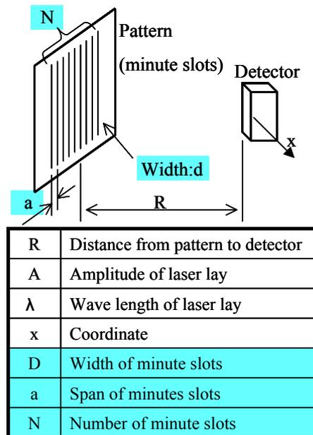
Fig.7 Parameters of Fraunhofer diffraction equation
