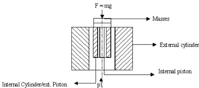
Fig. 1. Schematic view of the 500 MPa pressure balance
