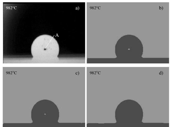
Fig. 3 Original image of specimen of silver (a) and results of its segmentation (b, c, d). (A – object removed in segmentation process)
