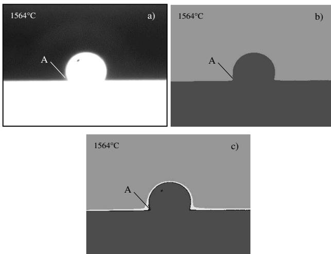
Fig. 5 Original image of specimen of palladium (a) and results of its segmentation (b, c).
