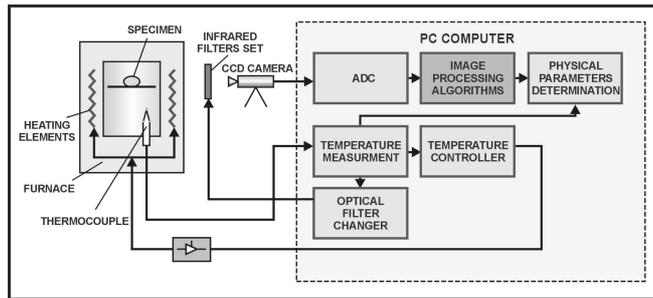
Fig. 1. Block diagram of computerised system with CCD camera for measurement of surface properties
