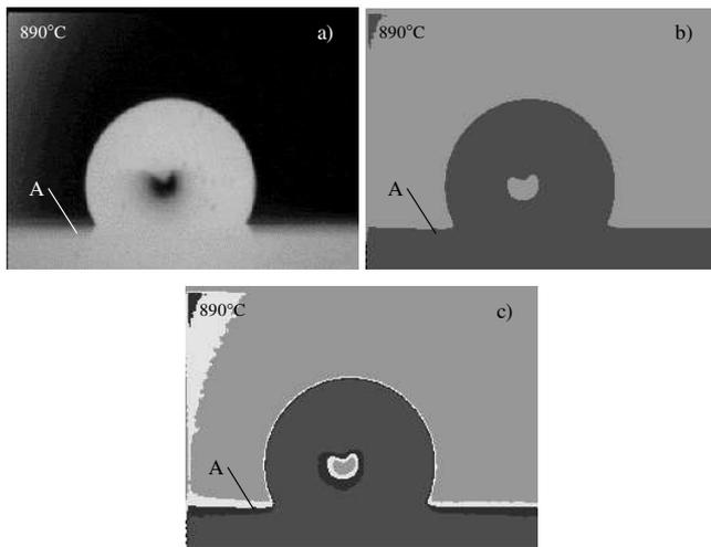
Fig. 4 Original image of specimen of glass (a) and results of its segmentation (b, c).
