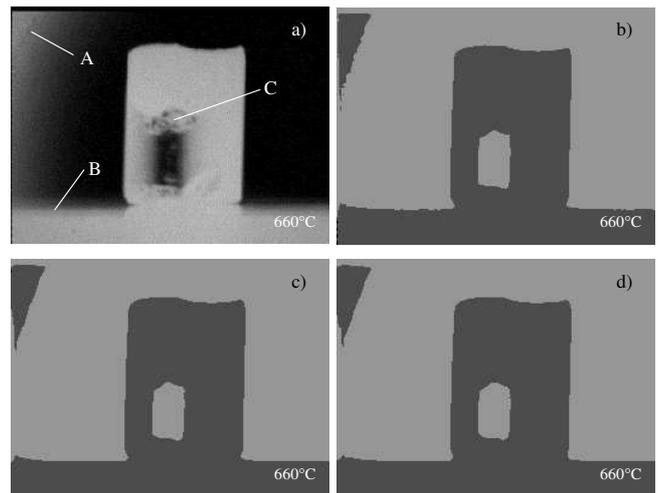
Fig. 2 Original image of specimen of glass (a) and results of its segmentation (b, c, d). (A – upper edge of the base-plate; B – fragment of internal foundry wall; C – object area with non-homogenous texture)
