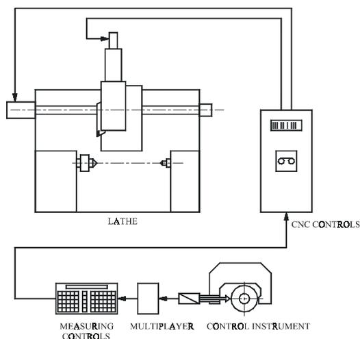
Fig. 1. Connection of measuring control unit with lathe control
