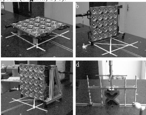
Fig. 2. Sequence of a plate positions assumed for determination of the reference grid: situation a) XY, b) YZ c) XZ in the consecutive position d) determination of FBG for the head.
