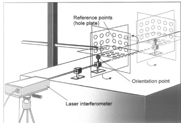
Fig. 4. The concept of transposing a matrix method for large machines
