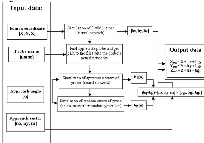
Fig. 3. Scheme of a virtual model based on neural networks [5]
