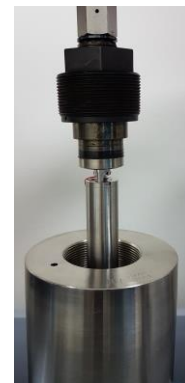
Figure 7: ultrasonic cell and high-pressure vessel (Imperial College London)
