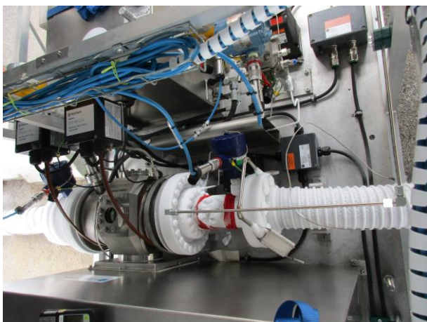
Figure 13: LDV standard for traceable cryogenic measurement (design and built by Cesame©) [12]
