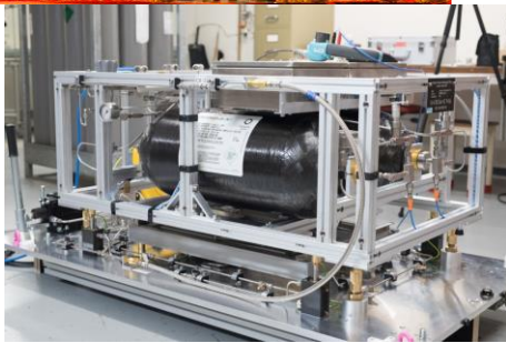
Figure 1: Gravimetric primary standard (design and built by METAS)
