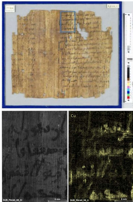
Fig. 5 Image of P. Hamb. Arab. 68.6r (top) indicating the area analysed; B/W image of the analysed section (left), and XRF map (relative intensity) of copper (right), using M6 Jetstream (Bruker nano GmbH).
