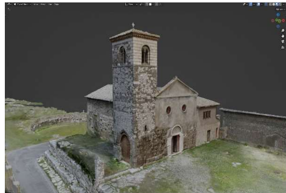
Fig. 1. View of the photogrammetric model of the church of S. Pietro in Segni in Blender.
