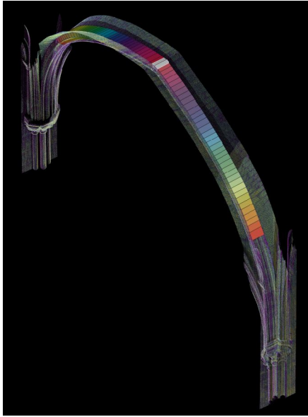
Fig. 3. An excerpt from the cathedral point cloud provides support for a parametric volumetric model of the arch with arbitrary colors. This image is technical and aesthetic.
