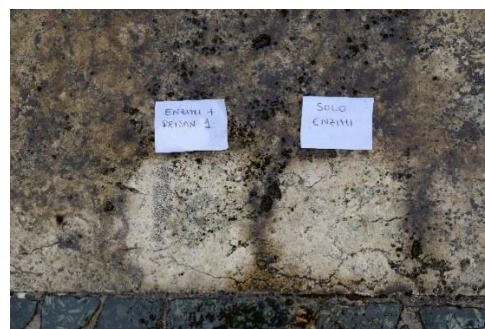
Figure 4. Area treated with only traditional enzymes in the matrix and area treated with both traditional enzymes and essential oils.
