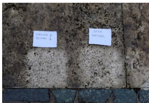
Figure 3. Area treated with only gel-based enzymes and area treated with both gel-based enzymes and essential oils.
