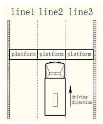
Figure 5: "Line pressing" driving
