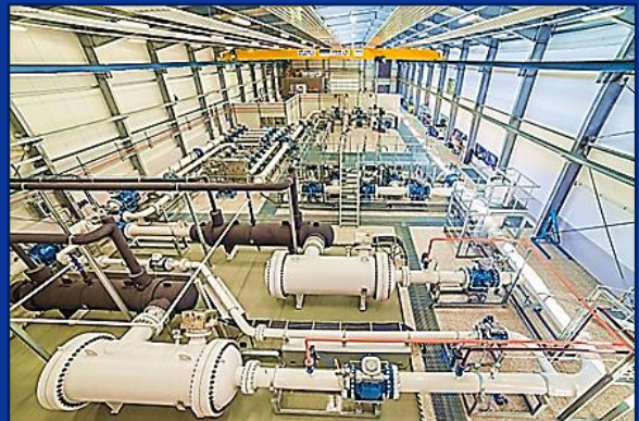
Worldwide First Bidirectional High Pressure Closed Loop Test Rig for Gas Meters (Medium: Natural Gas 5.5 MPa / 11.200m 3 /h).
